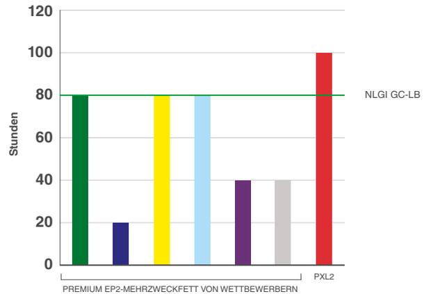
**ASTM D1742 ÖLABSCHEIDUNG**
