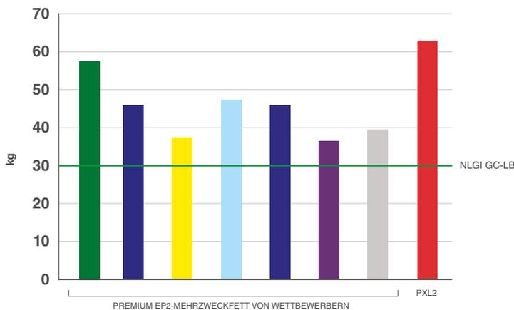
**ASTM D4290 RADLAGER-LECKAGE**
